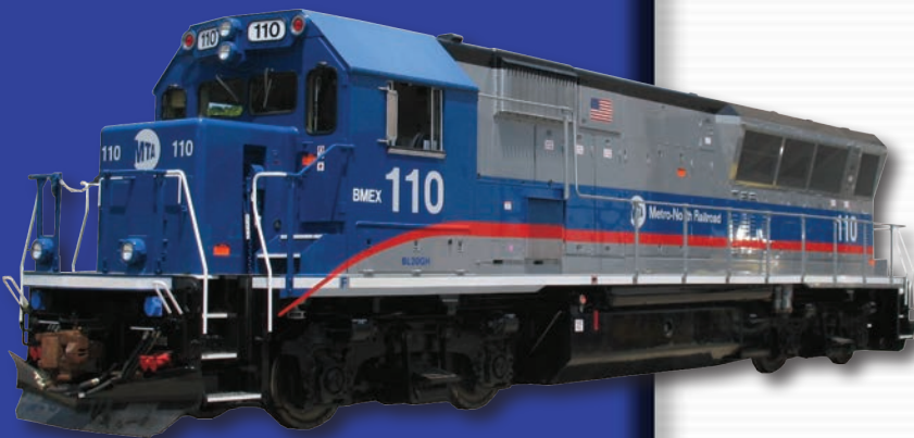
BL20GH 132 Ton - 2250hp Multi-Purpose Locomotive with Separate HEP
