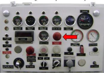
This Emergency Shutdown switch can be modified so it would not only shutdown the engine, it will also set the park brake in the event of its activation.
